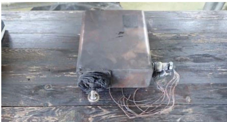
Foto 38: attuatore lineare del pitch trim ( Electromech Technologies 483-3 dual motor driven linear actuator ).
